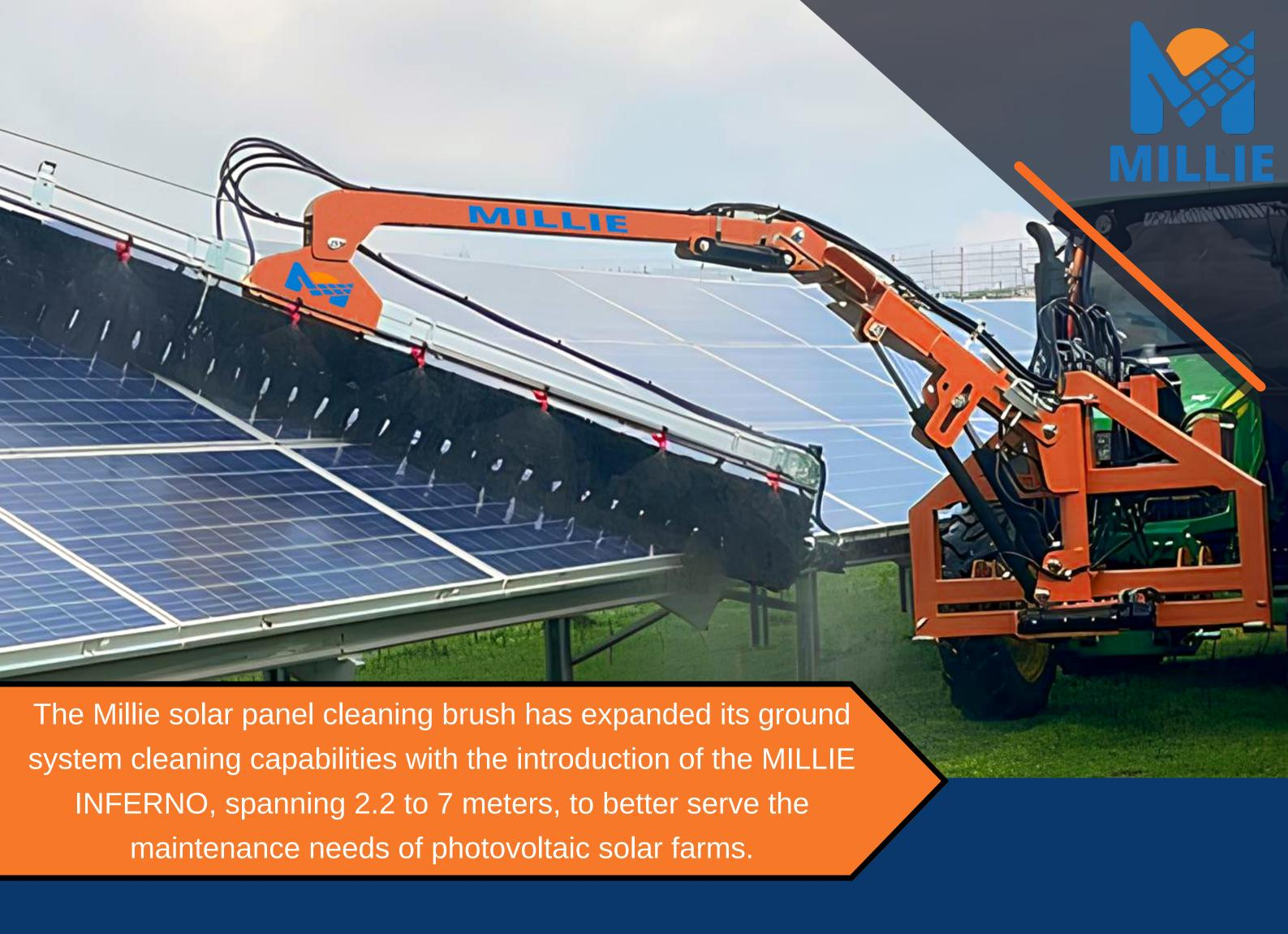
These cleaners can be effortlessly mounted on various standard vehicles like tractors, excavators, and telescopic loaders, providing exceptional mobility, straightforward installation, and effortless control. Optionally, Millie can be used in conjunction with a cleaning solution for your photovoltaic system, effectively working in both wet and dry conditions. It represents the next-generation product, meeting the diverse needs of operators.
